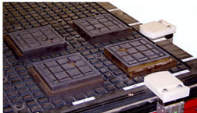
MOVING VACUUM PAD ◆ It may fix on any position of the table to absorb workpiece, and prevents aggregates from colliding with working table.
