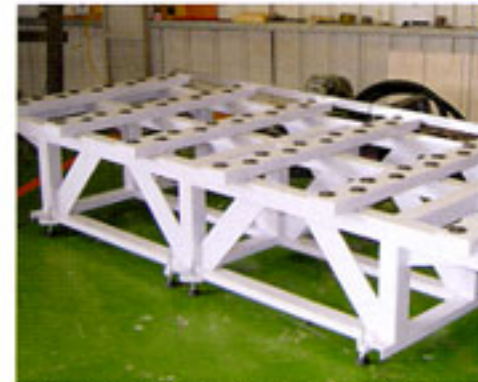
ROLLER CONVEYOR TABLES IN FRONT AND BACK OF MACHINE AND FLOATING TABLE TOP SYSTEM ◆ This can eliminate downtime for parts changing and also full board sheets can move more easily.
