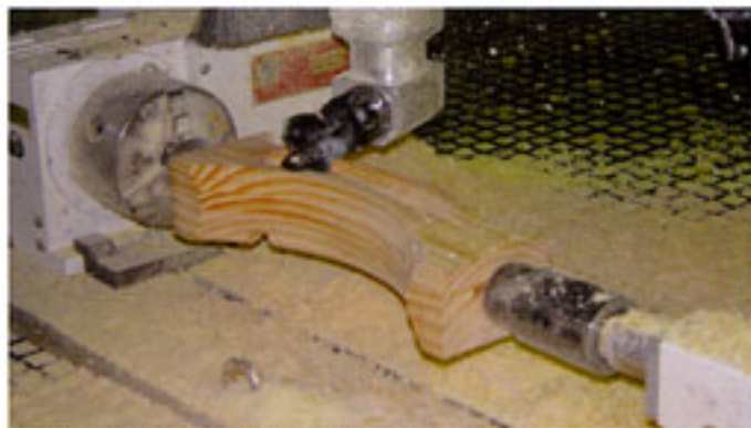
B AXIS WORKPIECE ROTARY MACHINING DEVICE ◆ Suitable for revolving cylinder type workpieces and stair handrails.
