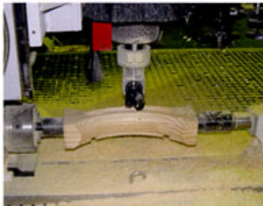
◆ PROCESSING STAIR RAILING
