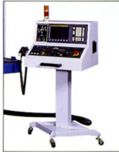
FANUC CNC Controller ◆ A Japanese brand CNC control
