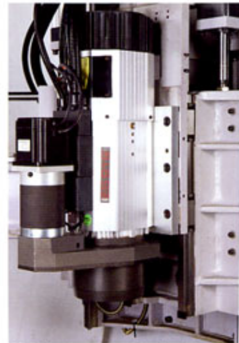
C-Axis Rotation Mechanism ◆ May process any angle between 0° ~ 360° for side processing and saw cutting.
