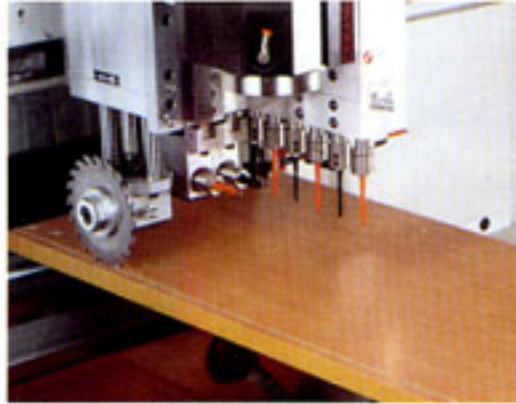
◆ Pneumatic line boring
