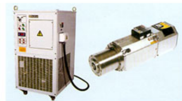
SPINDLE COOLING SYSTEM & HIGH FREQUENCY SPINDLE ◆ The circulated forced cooling system permits the spindle running at a constant temperature at all times, ensuring long services life of bearings.
