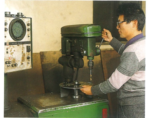
Blower fan balance test to ensure long service life of bearings, vibration free running and steady air flow.
