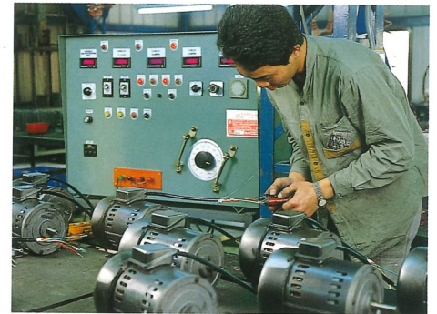
Motor performance test for current, voltage, and resistance.
