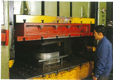
The blower casting is one piece, fabricated by a high performance hydraulic forming machine.
