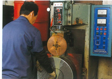
The blower casing is welded by a seam welding machine to ensure uniform welding result and a smooth welding surface.
