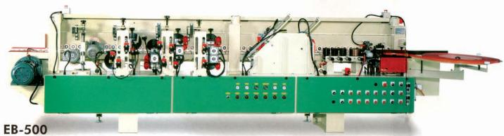
Veneer Infeed>Coil Cut-off>Gluing and Press>End Cutting>End Trimming>Fine Trimming>Scraping>Buffing
