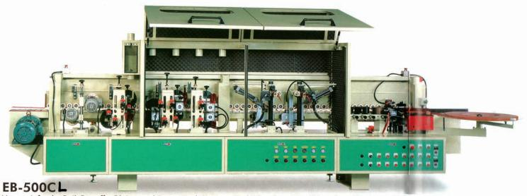
Veneer Infeed>Coil Cut-off>Gluing and Press>End Cutting>End Trimming>Fine Trimming>Scraping>Buffing
