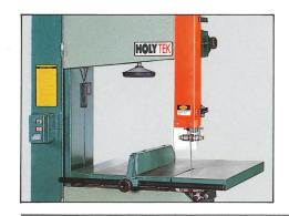
The tension blade indicator indicates the blade tightening and reduces the breaking risks.
