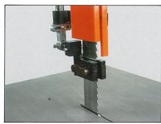
Bakelite fitted on the blade guide assembly gives extra rigid side support. Special for model HB-600, 700, 800, when a wide blade is applied.
