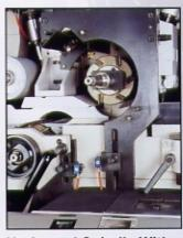
Horizontal Spindle With Jointer Device (Optional)
