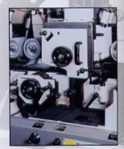
Hydraulic Clamped Outboard Bearing System (Optional)
