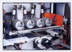
Powered Upper and Lower Feed Roller and Pneumatic Side Pressure Wheels
