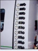
Individual Adjustable Pneumatic Pressure Gauges for Different Pneumatic Control Units
