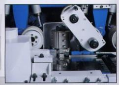
Vertical Spindle Adjustment up to 80 mm
