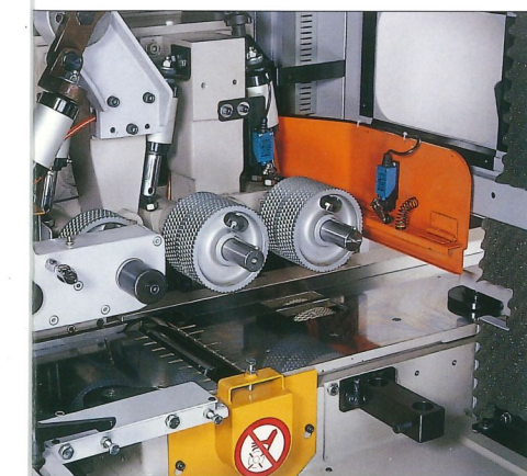
UPPER AND LOWER INFED WITH PNEUMATIC CONTROL Rollers are powered, providing pneumatic control and a pressure gauge for a smooth feeding effect. A limit switch provides protection from oversized stock.
