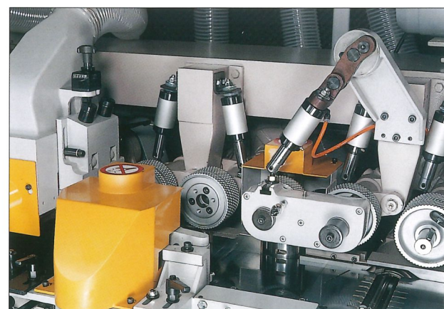
SIDE FRONT PRESSURE PLATE ON LEFT VERTICAL SPINDLE WITH ADJUSTABLE TABLE Eliminates smoothness problems when feeding short or narrow stock. The pressure plate is easy to adjust. The vertical spindle table can be adjusted to suit different cutter diameters.
