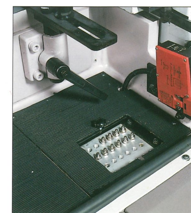
CENTRALIZED LUBRICATION The spindles are lubricated by the centralized lubrication system for convenience.
