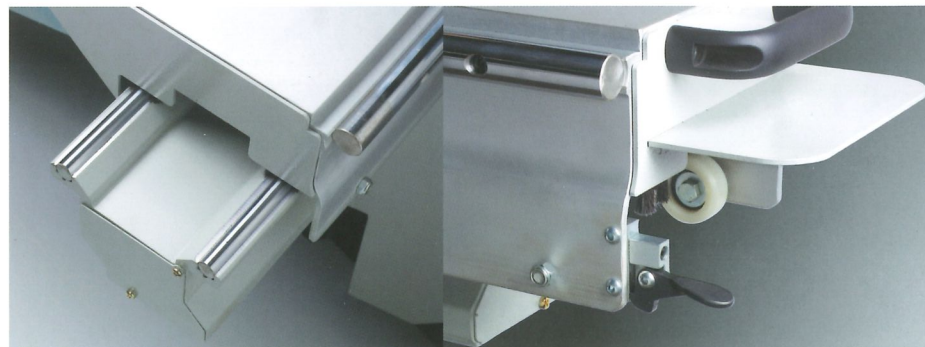
Sliding Table The multi-chamber sliding table is manufactured by a highly reputed European aluminum company. It also features a built-in wheel-type sliding mechanism. The rail is manufactured from high-tensile steel, heat treated and the surface is chrome plated for lifetime straightness.
