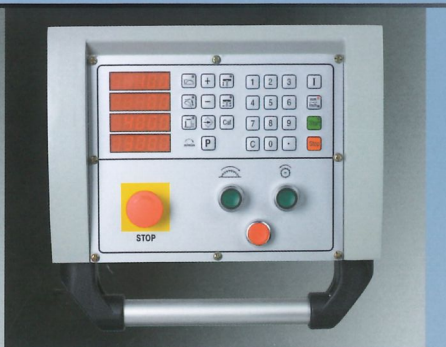
CNC Control Panel The standard fixed or optional hanging-type controls can be used for setting the saw blade up or down, tilting and cutting width dimensions. Also, there is a 30-set of program memory capacity.
