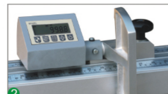
2 Digital display on the transverse guiding ruler
