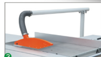
3 Simple dust sucking device
