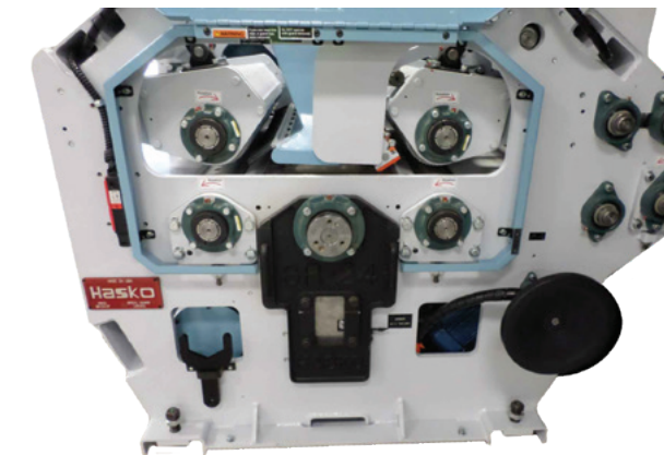
Robust design and simplicity include “Quick Clear” function for raising feed rolls
