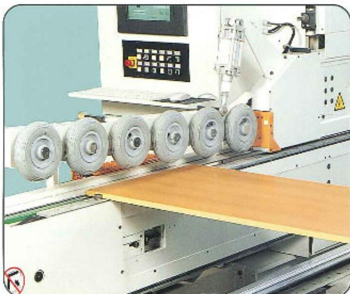
*During automatic crossways machining, a sophisticated centring system always guarantees piece alignment against the machining line.*
