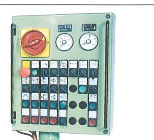
panel positioned at the infeed of the machine in a suitable ergonomic position.
