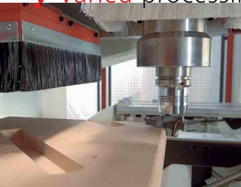
Drilling ① [14 + 6 spindles]
