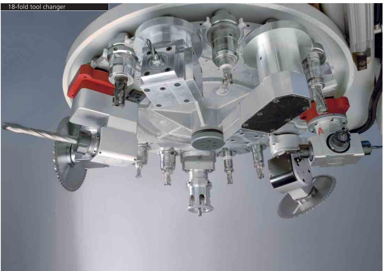
2 B Drilling ② [21 spindles]
