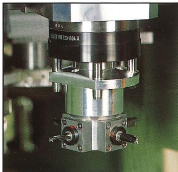
**Adapteraggregat, Horizontalbohrer,** 4-spindlig,
