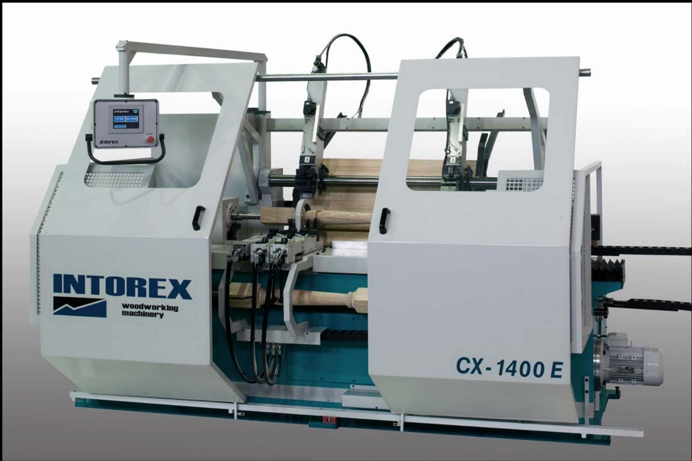
Fully automatic electronic lathe equipped with 2 hydraulic copiers and 2 form tool sets
