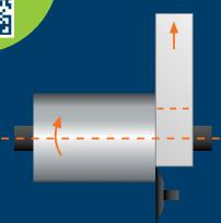
Slitting unit with circular knife for dividing the roll on the pay-off shaft.
