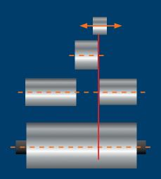
Positioning of roller cutters by means of the laser guide light.
