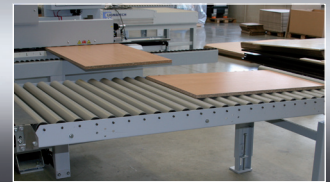
Leaving-side roller track
