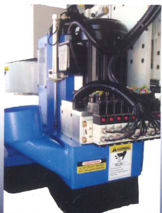
Individual pneumatic valve for each drill
