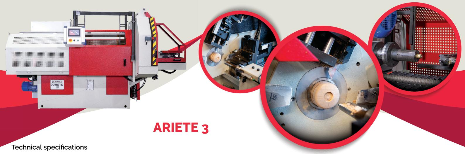
Fully automatic hydraulic lathe with feeder, fitted with clamping device for a perfect centering of the wooden blanks, ideal for the production of small timber components made from square stocks. The headstock runs on linear guides and is driven by a brushless motor with ball screw and
