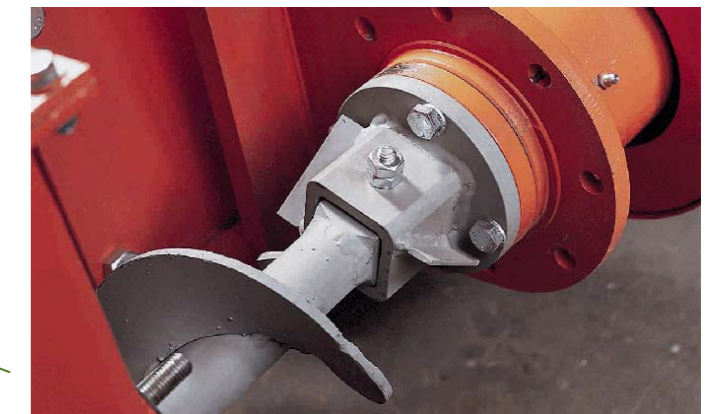
Screw pivots around a universal joint on one end thereby allowing the screw to avoid oversized pieces inside the pipe housing
