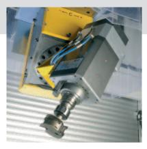
**Routing unit**with tool interface HSK F 63,
