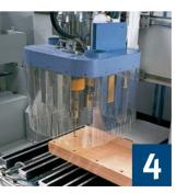
Dust and chip collecting basket mounted to the routing unit, vertically adjustable via CNC
