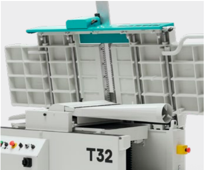
T32 equipped for thickness planing mode
