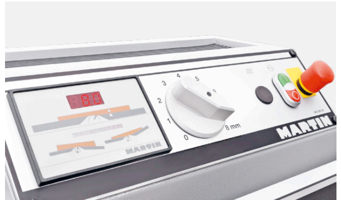
Control panel combined with and moves with surfacing fence | T544
