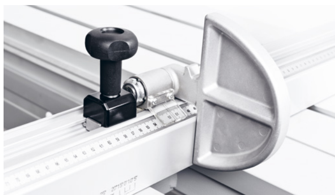
Length compensation in angle cuts | Standard
