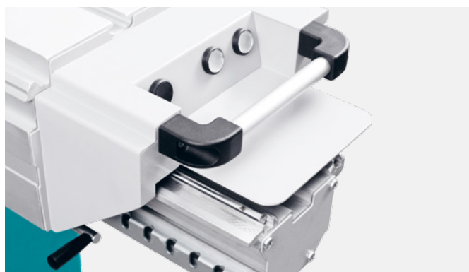
Sliding table on switch | TC66x285
