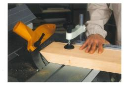
Tilting saw unit with a 250 mm blade and a maximum cutting depth of 80 mm. The saw will cut panels 500 mm wide at the rip fence.
