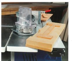
**Spindle moulder guard** for moulding shapes and curved profiles.
