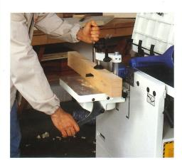
Slots, recessing and mortise and tenon joints are easy with **the slotter unit**.
