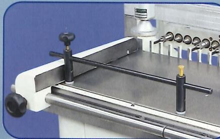
Reference fences for precise boring operations and mechanical gauge\* for a perfect symmetry.
