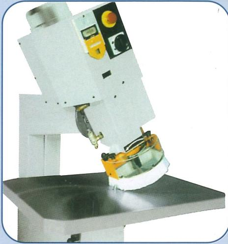
The tilting head allows boring, routing and tilting shaping up to 45°, to the right or to the left of the vertical axis.
