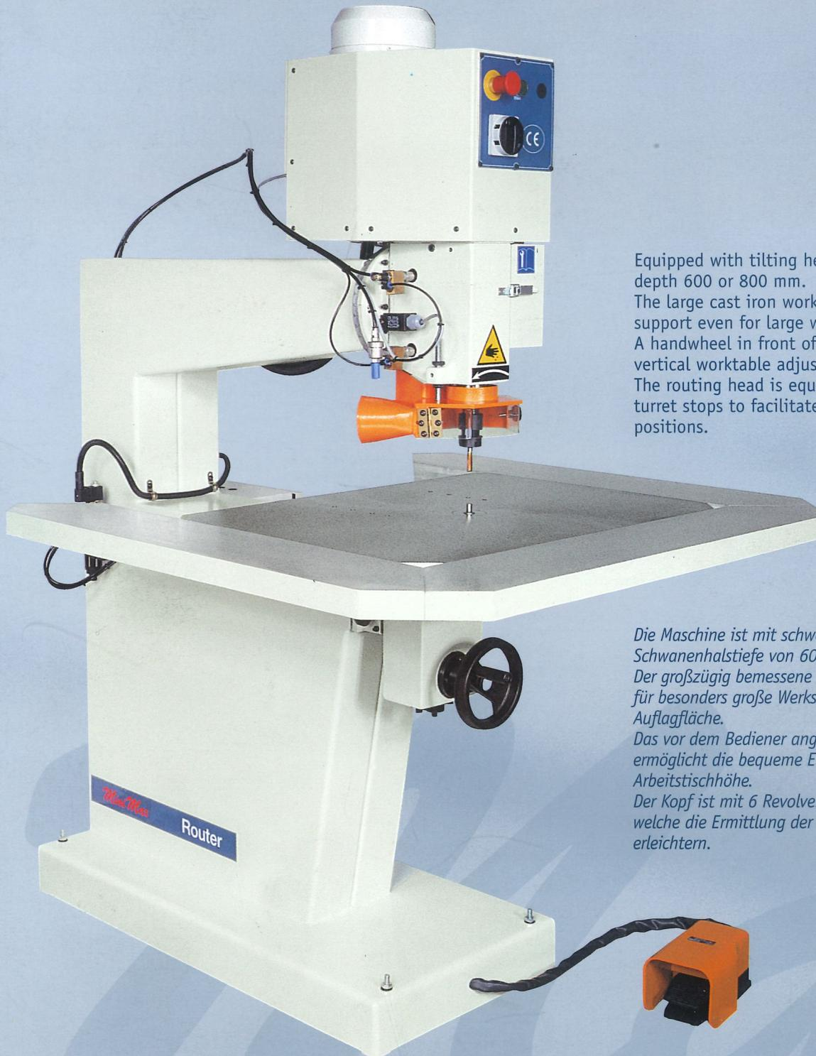
Equipped with tilting head with neck depth 600 or 800 mm.
