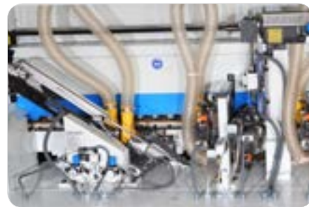
YENİ BAŞ-SON KESME NEW FRONT AND BACK CUTTING UNIT
