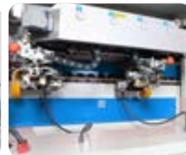
AÇILI ÖZELLİKLİ BAŞ-SON KESME ANGLE ADJUSTABLE FRONT AND BACK CUTTING UNIT
