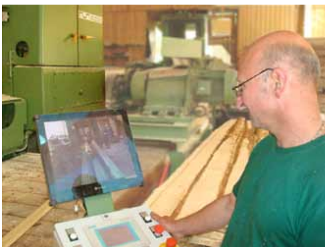
Fully-automated frame saw operation
