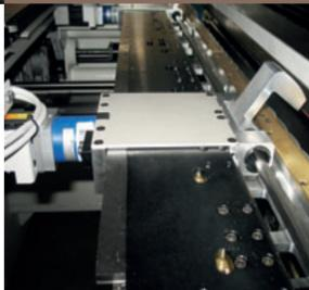
Work tables with independent movement and positioning in relation to the lower drilling units: the best optimisation of the machine work configuration allows the user to move the drilling units during machining without restrictions and risks to the panel surface coating
