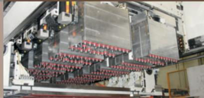
Complete in all its operations: possibility of inserting a specific unit for hinges on every lower machining head and on every upper head a specific unit for the horizontal drilling in Y (longitudinal).
