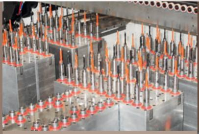
Multitude of configuration choices for every type of requirement and level of investment: up to 6 upper units and 6 lower units with two drilling heads each, for a maximum of 24 drilling heads.
