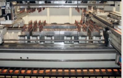
The most flexible solution which can be applied in the creation of your workpieces: the automatic and independent rotation of every drilling head, also within the single machining program, ensures utmost efficiency also with complex drilling patterns.
