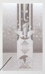
Hollow chisel mortising involves a special drill revolving inside a hollow square chisel. The drill makes a pilot hole and the chisel finishes the mortise by removing the area around the hole leaving a straight sided square mortise.
