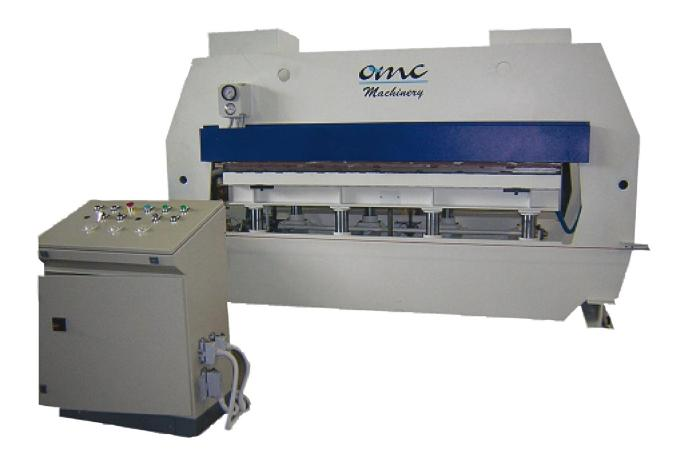
This press is right to cover ashlars and doors with veneer on both sides. The inferior movable plate is guided by a series of crossed racks. Solid and perforated plates with iron frame to fix the membrane. The Fluid press has a liquid pouring off system by a high capacity pump. The press is fitted with a double membrane always in contact with the heated plate also during still work. A cut flamed structure guarantees a great stability at a high quality work. No extraction tray.
