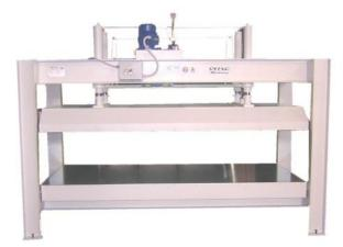
This cold press model has chipboard plates covered with galvanized iron sheet, movable superior plate from top to down.
