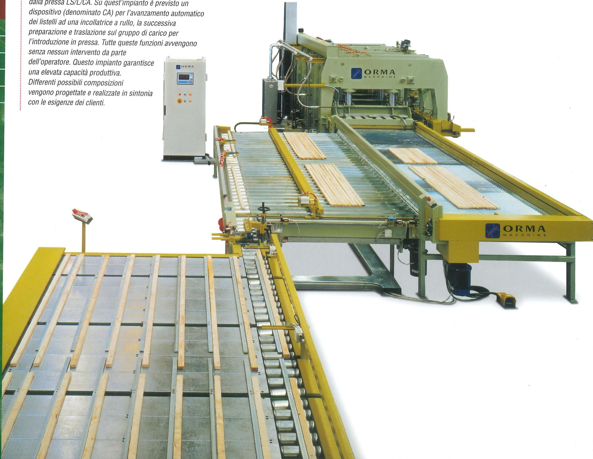
*LS/L/CA is a further evolution of the LS/L type. This line foresees a device (named CA) which allows the automatic feeding of the boards through the one roller glue spreader, their transfer and laying up onto the loading table from which will be pushed into the press. All these steps are automatically controlled and do not need the operator action. This plant grants a high output. Possible different lay outs are designed and manufactured in accordance with the customers' needs.*
