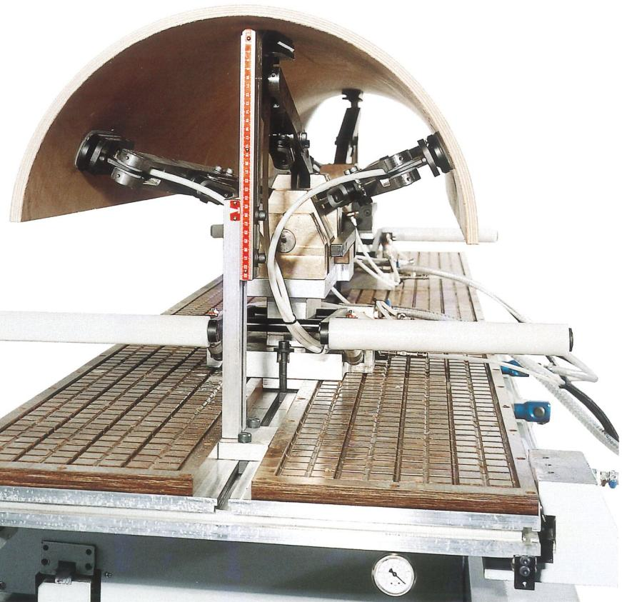
**E**quipment for blocking curved components with easy and rapid adjustment. TRIX avoids the necessity to prepare fixing jigs with enormous cost saving in both equipment and time. It consists of a system of multiple expansion arms each with mobile pneumatic suction cups for vacuum blocking. It is adjustable in basis of the size of the component to be machined. Its roller system aids the loading / unloading and positioning of the work components.
