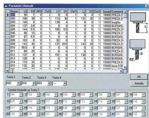
**D**edicated interface with teach-in programming and management of work cycles. The teach-in system allows the operator, by a remote control, to move the 5 axis of the machine and incline the head in the position where a certain operation will be made (tenon or mortise, holes, etc). It is very useful when programming starting from a sample piece.
