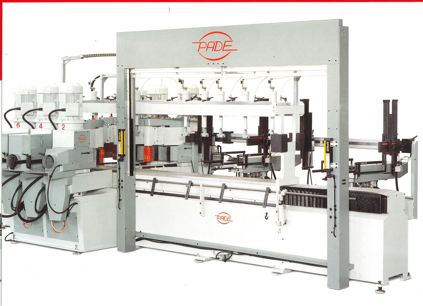
**Opening of one side of the machine (models UINZE 6T and 8T CNC) for an easy and full access to tool change area: a hydraulic device with automatic levelling will activate rapidly and precisely the opening and closing of the unit. Completely mechanical system for the oscillation of the sanding paper. Pneumatic holdown clamps with hexagonal shaft and antirotation system.**
