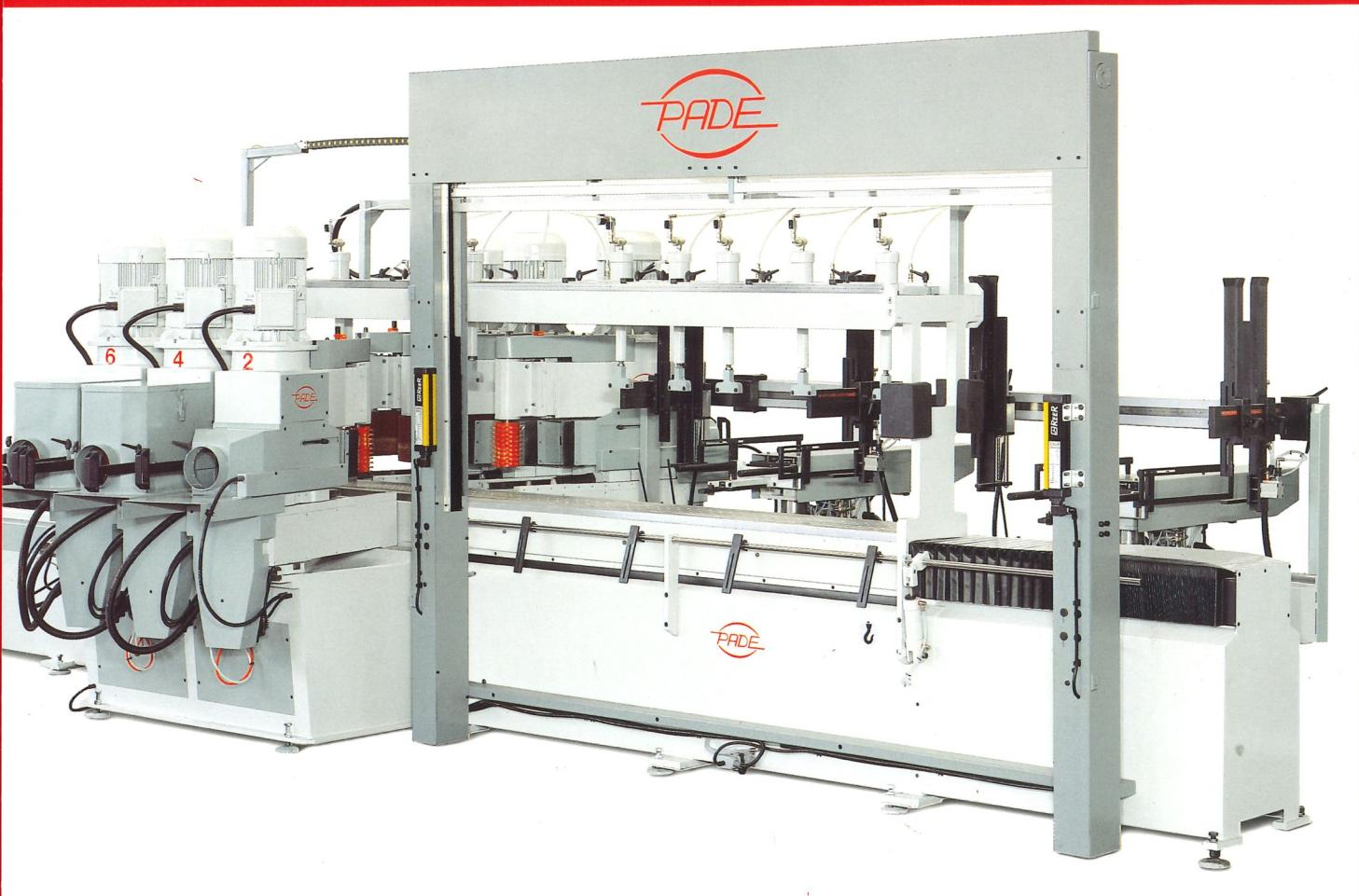
**Sturdy and rigid construction. Absolute precision and maximum reliability. Working head tilting at -10° 0° +10°, motorized positioning controlled by the CNC. No template needed. Complex profiles such as double rounding at both ends of a workpiece can be executed. Return speed of the table at 90 mt/min without slowing down along the stroke.**
