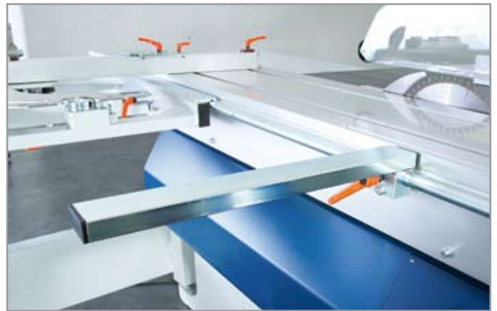
Additional support for large panels
