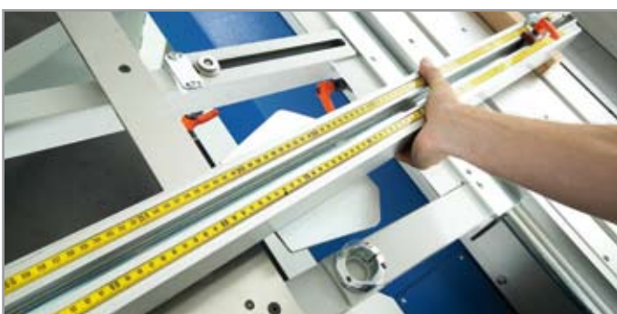
Comfort clamping for crosscut fence self-stopping, tool-less connector system
