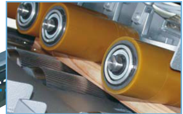
Fig. 12: Wide feed rollers ensure optimum timber guidance in the cross-cut station
