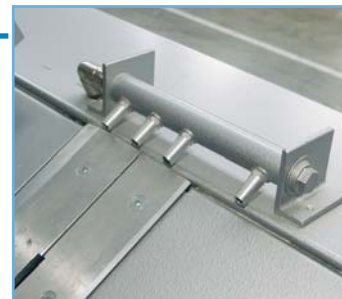
Fig. 13: Air-jet blower in the cutting area
