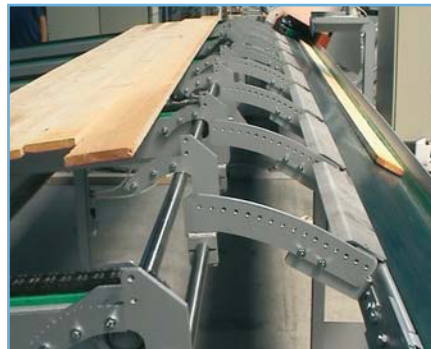
Fig. 20: Buffer feeding system
