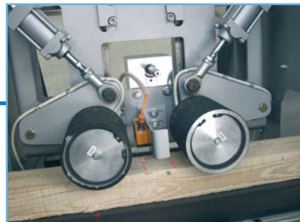
Fig. 7: Crayon mark recognition in measuring station
