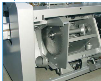
Fig. 14: The saw blade is completely enclosed and easily accessible
