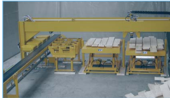
Fig. 19: Pneumatic ejectors followed by an auto stacking and destacking system
