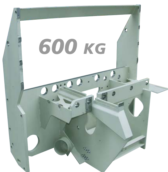
Fig. 3: The bare steel frame weighs 600 kg
