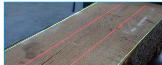
Fig. 3: Line lasers for accurate workpiece alignment
