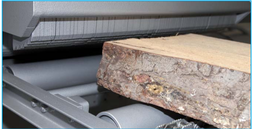
Fig. 9: Anti-kickback device for increased safety
