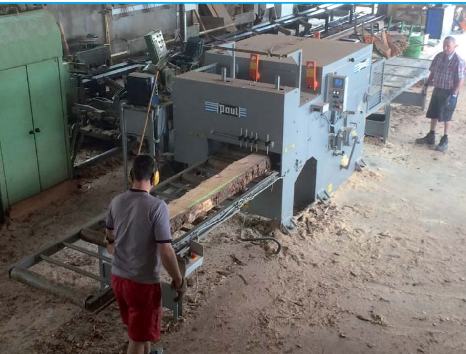
Fig. 2: S-918, manually loaded, with infeed pinch roller unit, operating in a sawmill
