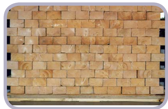
Fig.2: Offset layers for increased stability
