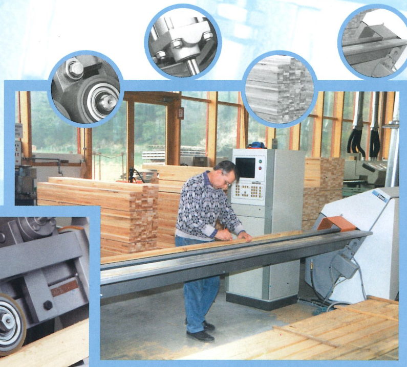
Fig. 8: Defect marking on model 11KE
