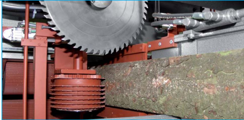
Fig. 18: Slab extractor with slab cross-cut saw
