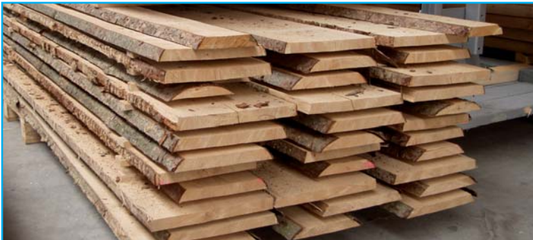
Fig. 6: From waney-edged boards ...
