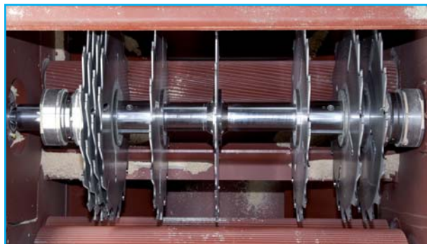
Fig. 11: Telescopic saw bush configuration for ripping into 4 variable finished widths
