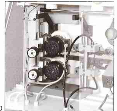
10) 2-motor buffing unit for cleaning and polishing of plastic edges (2 x 350 W 3.000 rpm).
