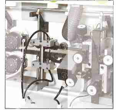
9) Self-adjusting glue scraper for cleaning of flat surfaces.
