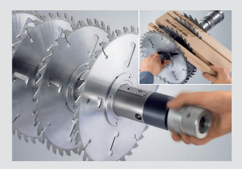
Less set-up, more ripping! With RAIMANN's patented Quickfix saw arbor system, saw blades can be clamped directly on the arbor (minimal dimension between blades is 25mm). No sleeve, no spacers, no tools! All saw blades are easily adjusted by hand. The result: flexible ripping, huge timesavings. Set-up in less than a minute!
