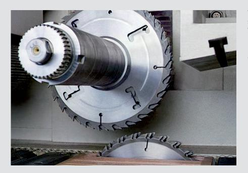
The KRD 310 uses the narrowest kerf saw blades ensuring best possible yield. This machine is ideal for cutting material up to 180 mm thick. With its accurate material transport, a precise cut is guaranteed.
