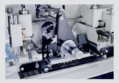
The moving pressure shoe segments, synchronous with the moving blades, ensure superior board control during the cutting process. Even outer edges are securely held down during ripping and transported safely out of the machine. Ripped pieces cannot lift up, so throughput is not interrupted. Optimal material hold-down means better quality of cut.
