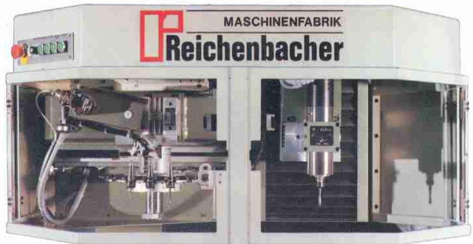
The tools are fixed with a precision taper ATC 16. The automatic tool changer with 16 positions ensures the use of different cutting tools.
