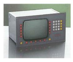
The functions of CONTROL 5.0 are selected directly via softkeys around the screen.
