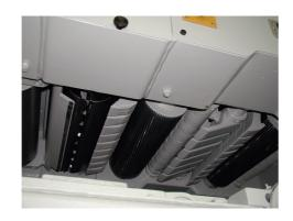
Conventional narrow machines are only fitted with feed rollers mounted on one side which cannot guarantee problem-free workpiece transport.
