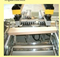
Drilling from top, back and ends. in the picture you see asymetric details drilled.
