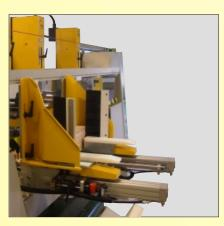
Components are fed in, held in position and ejected by pneumatic clamps, thus ensuring positive feeding without marking the timber.
