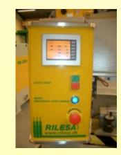
The control system is easy operated from the touch screen display, with options as cross drilling, and cleaning of drill holes etc.
