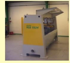
The machine is equipped with a large door on the backside, it gives easy access to the drilling groupes.
